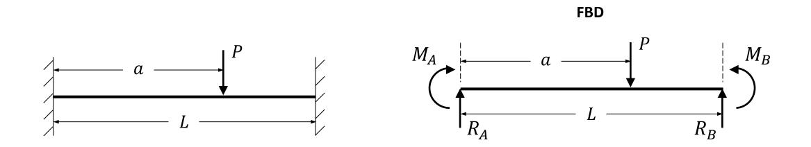
Taking the left-hand end as the origin and drawing a free body diagram of the beam sectioned after the discontinuity:
