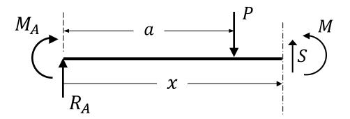
Taking moments about the section position in order to determine an expression for the bending moment, M:
